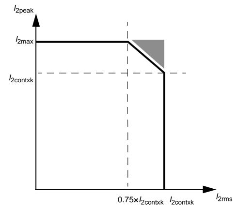
The above procedure can also be applied to longer load cycles by dividing the cycle into subcycles no longer than 10 seconds. If any of the subcycles fail the test, a more detailed study is required.
